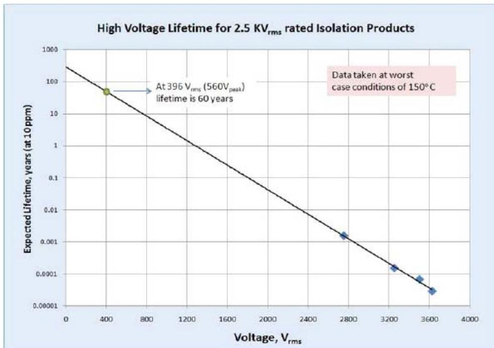
Figure 10. ILX488-3 Time-Dependent Dielectric Breakdown
