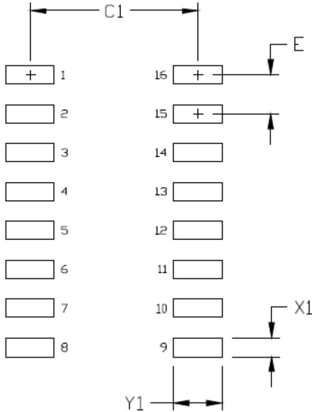
Figure 12. 16-Pin Narrow Body SOIC PCB Land Pattern
