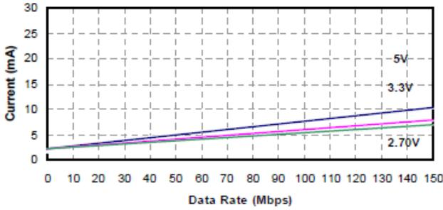
Figure 7. Si8431 Typical VDD1 Supply Current vs. Data Rate 5, 3.3, and 2.70 V Operation
