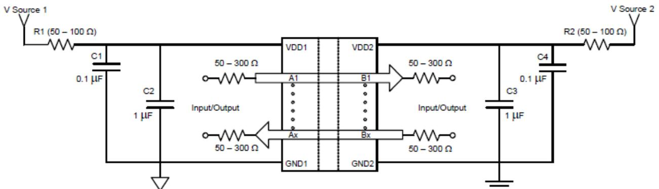
Figure 6. Recommended Bypass Components for the ILX488-3 Digital Isolator Family
