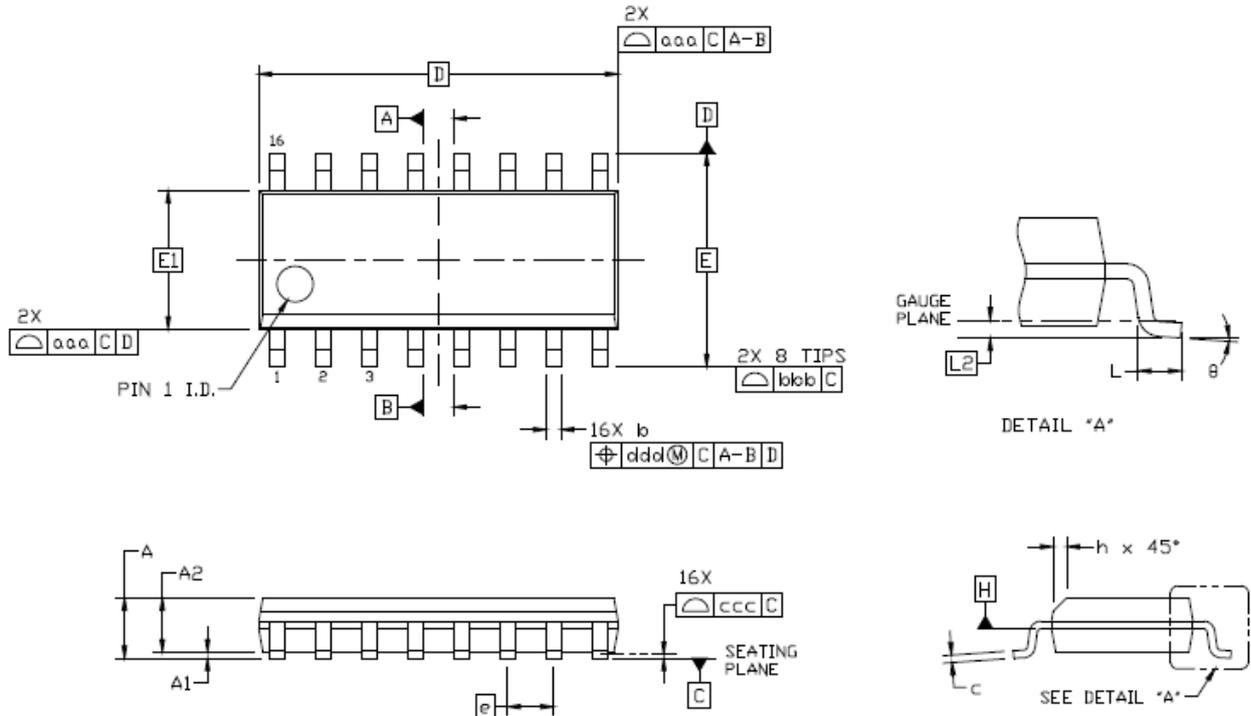
Figure 11. 16-pin Small Outline Integrated Circuit (SOIC) Package
