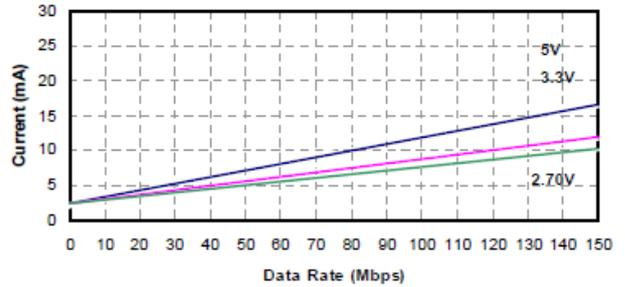
Figure 8. ILX488-3 Typical VDD2 Supply Current vs. Data Rate 5, 3.3, and 2.70 V Operation (15 pF Load)
