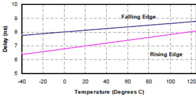
Figure 9. Propagation Delay vs. Temperature
