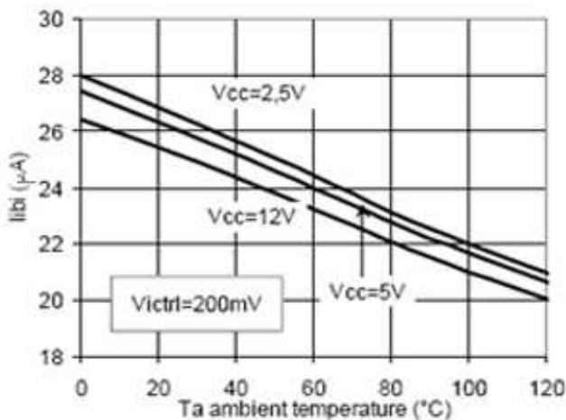
Figure 11: Supply current vs Ambient Temperature
