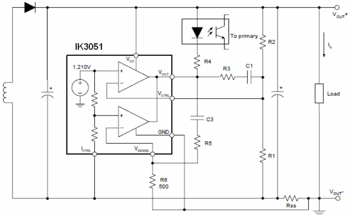
$$V_{OUT} = [V_{REF} + (I_L \times R_{SS})] \times \frac{R1 + R2}{R1} - (I_L \times R_{SS}) \quad (V)$$
