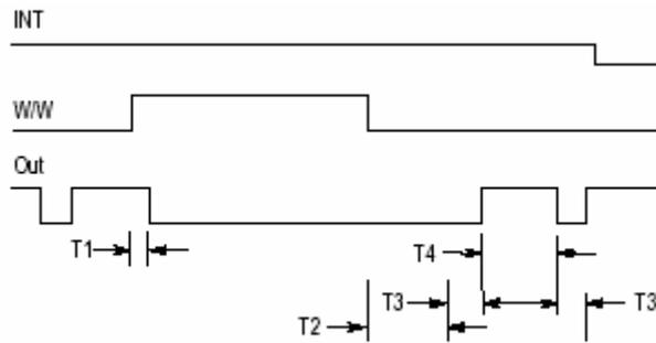
Figure 4. Switching Waveform W/W and INT Active
