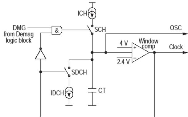
Figure 5. Oscillator Block
