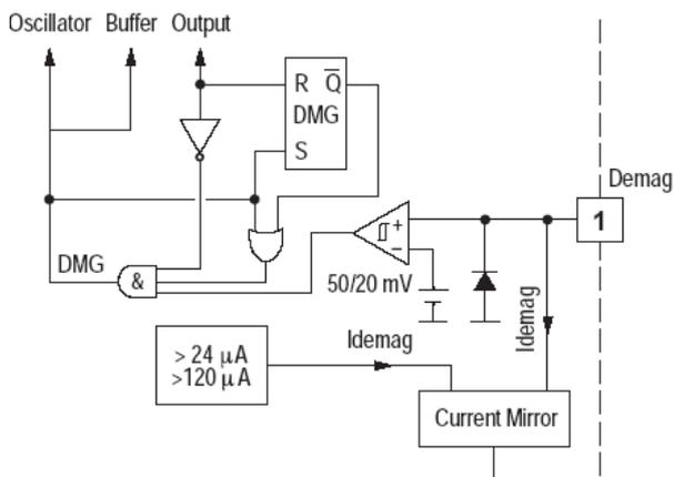
Figure 4. Demagnetization Block
