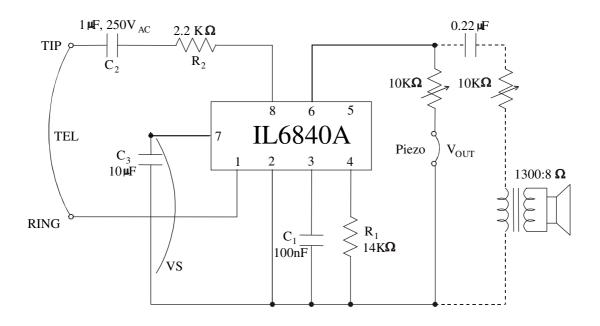
$$f_1 = 3.22 \bullet 10^4 / R_1 (K\Omega); f_2 = 5/7 f_1; f_{sweep} = 1000 / C_1 (nF)$$
