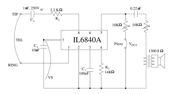
$$f_1 = 3.22 \cdot 10^4 / R_1 \text{ (K}\Omega); \quad f_2 = 5/7 \text{ } f_1; \quad f_{sweep} = 1000 / C_1 \text{(nF)}$$
