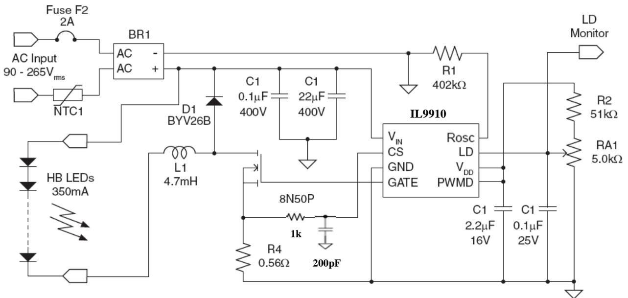
Figure 3. Typical Linear Dimming Application Circuit
