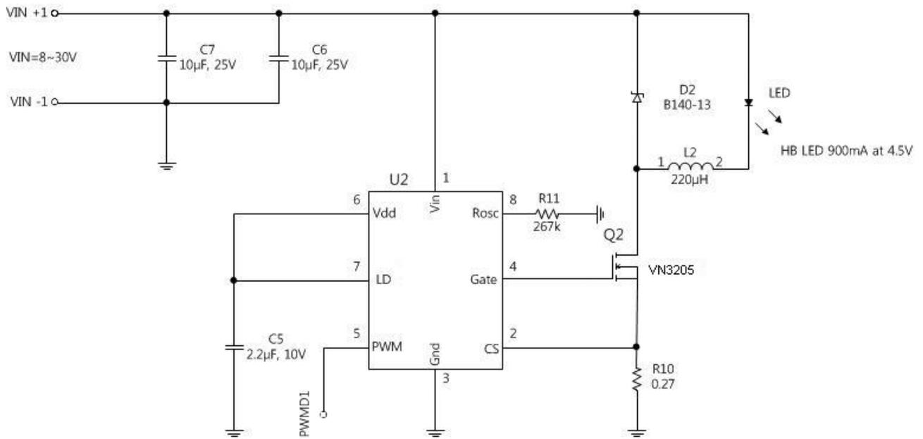
Figure 4. IL9910 Buck Driver for a single 900mA HB LED ( $V_{IN} = 8 \sim 30V$ )
