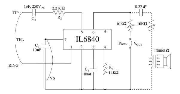
$f_1 = 3.22 \bullet 10^4 / R_1 (K\Omega); f_2 = 5/7 f_1; f_{sweep} = 1000 / C_1(nF)$
